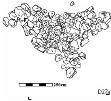
Figure 3.34. Collapsed wall stones and voussoirs above Rooms 617 and R603.
